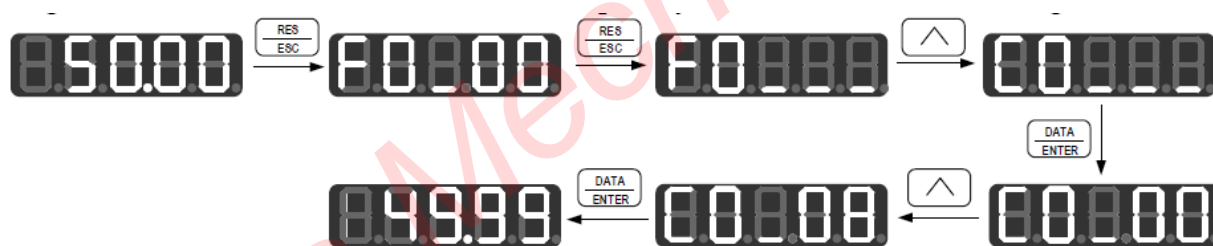
Figure 4-7 Procedures for Viewing and Editing Operation Monitoring Parameters
